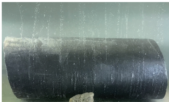
图9 普陆页1井千一段泥页岩中页岩气沿裂缝溢出照片 Fig.9 Photo of shale gas emission from micro fractures of shale in the first member of Qianfoya Formation in Well Puluye 1
